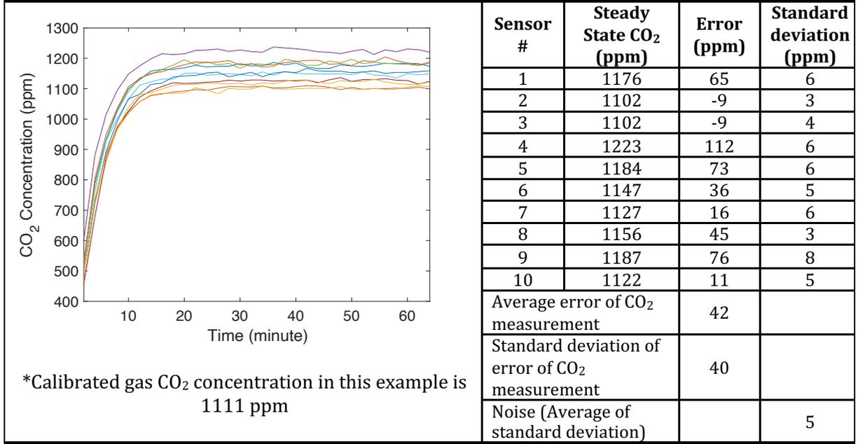
Figure 2.3: Illustration of an example test of the steady state average, standard deviation, and noise for each sensor.
