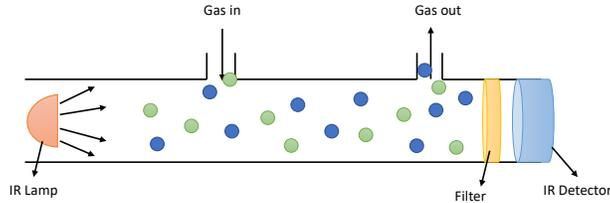
Figure 1.1: Non-dispersive infrared (NDIR) CO<sub>2</sub> sensor.
