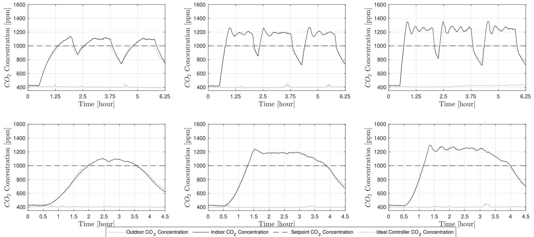
Figure 3.8: The outdoor, indoor (chamber), and ideal controller CO<sub>2</sub> concentrations for the Manufacturer 4 DCV test with the gradual (top) and step (bottom) generation profiles for low, medium, and high occupancy densities (left to right).
