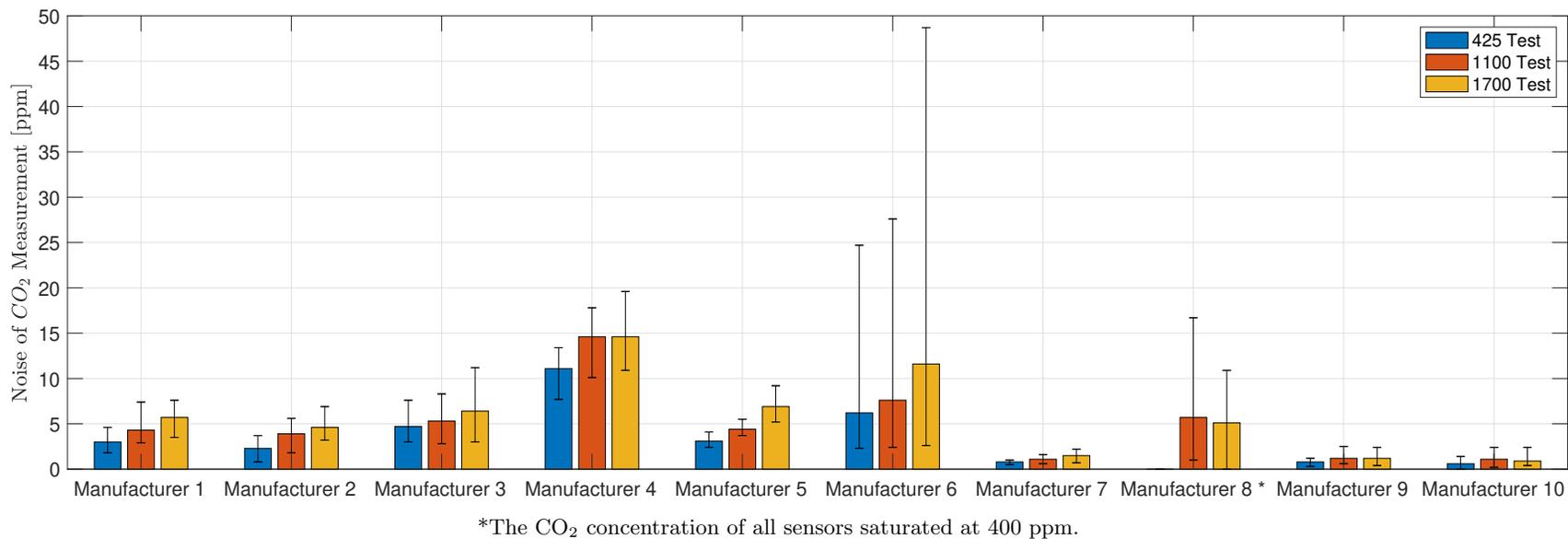
Figure 2.5: The average noise (i.e., average standard deviation over all ten sensors) for each sensor model and calibrated gas tested. The error bars represent the full range (minimum to maximum) of the standard deviations observed across the ten sensors tested.
