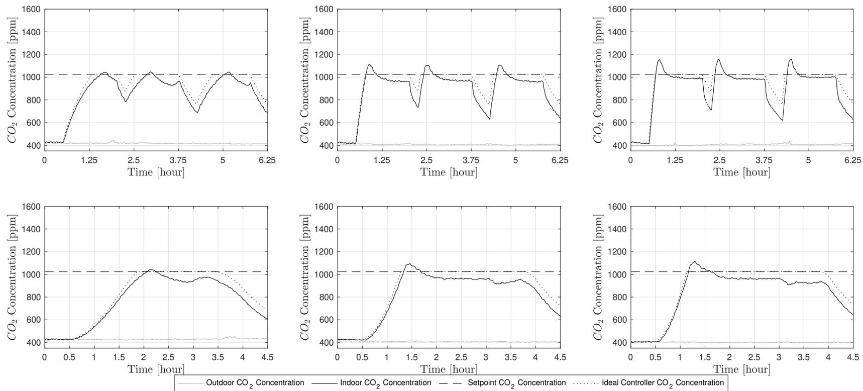
Figure 3.5: The outdoor, indoor (chamber), and ideal controller  $CO_2$  concentrations for the Manufacturer 1 DCV test with the gradual (top) and step (bottom) generation profiles for low, medium, and high occupancy densities (left to right).
