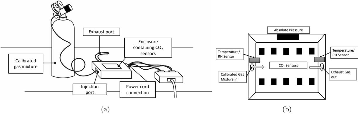
Figure 2.1: (a) An overall diagram of the experimental setup of the CO<sub>2</sub> sensor test protocol and (b) a diagram of the enclosure with ten sensors.
