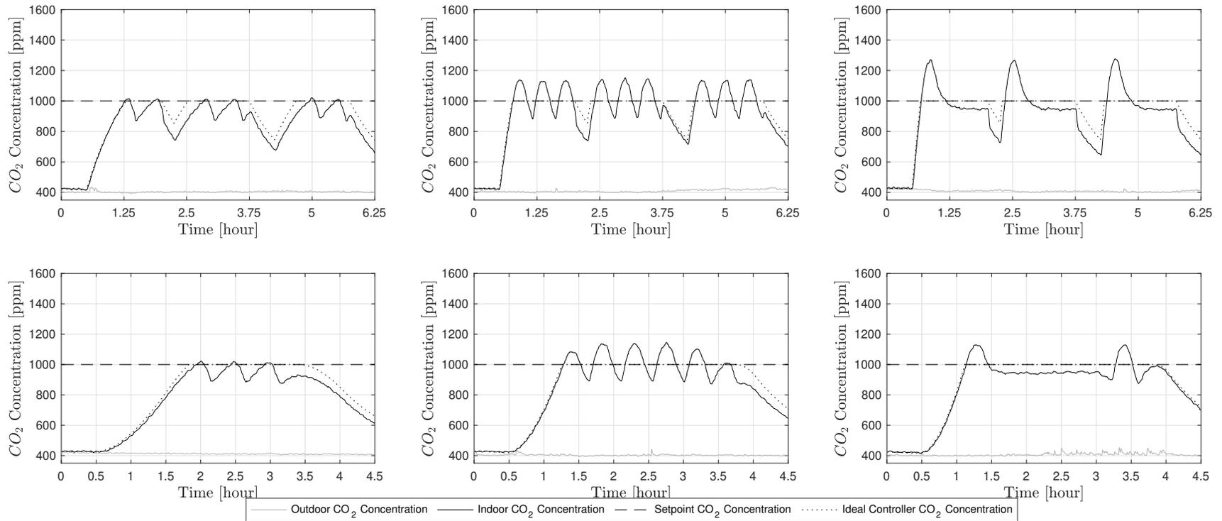
Figure 3.6: The outdoor, indoor (chamber), and ideal controller CO<sub>2</sub> concentrations for the Manufacturer 2 DCV test with the gradual (top) and step (bottom) generation profiles for low, medium, and high occupancy densities (left to right).
