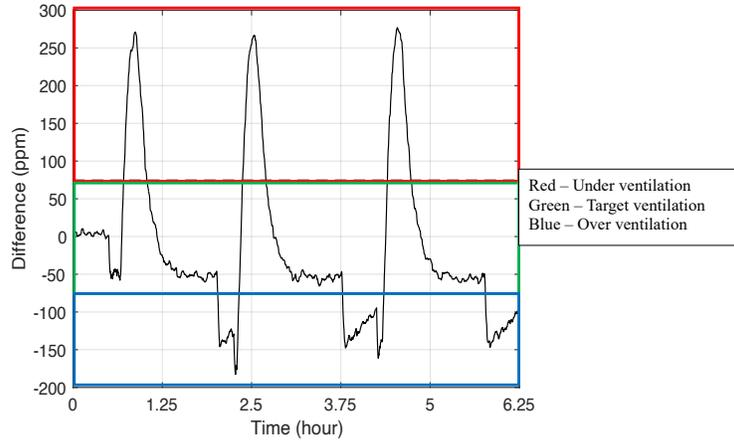
Figure 3.4: An illustration of the categorization that the controller under ventilates, over ventilates, and ventilates within the target is determined. The boxes highlight the times during the test that the controller is under ventilating, over ventilating, or at the target ventilation.
