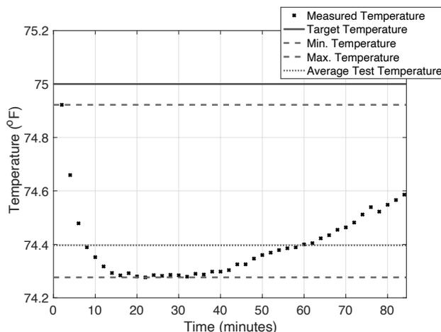
Figure 2.2: Illustration of an example temperature measured during a test with the two tolerances that must be satisfied during the test.
