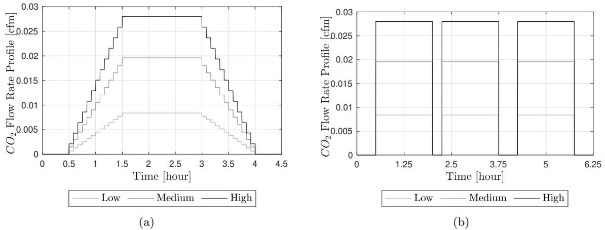
Figure 3.3: CO<sub>2</sub> generation rate for (a) a gradually changing occupancy profile and (b) a series of step changes in the occupancy for three occupancy densities.
