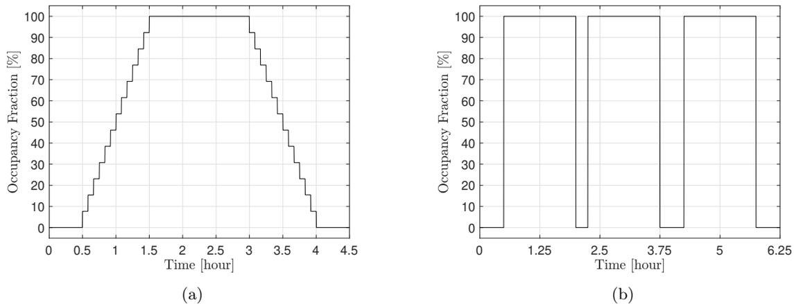
Figure 3.2: Occupancy fraction ( $Occ_{frac}(t)$ ) for (a) a gradually changing occupancy and (b) a series of step changes in the occupancy.
